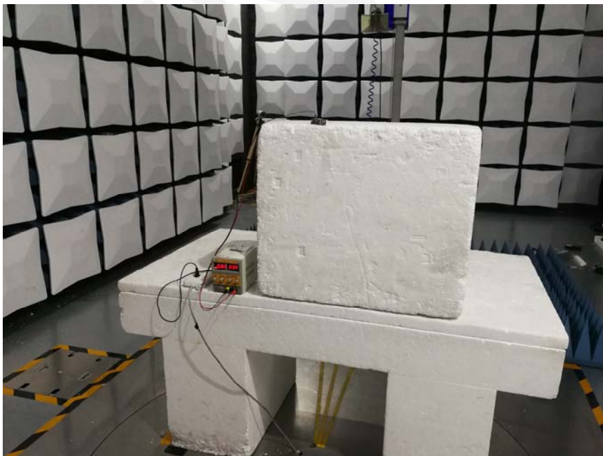
Radiated Spurious Emissions Test View (Above 1GHz)
