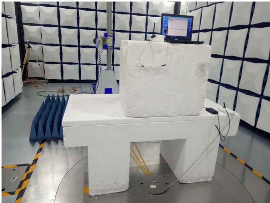
Radiated Spurious Emissions Test View (Above 1GHz)
